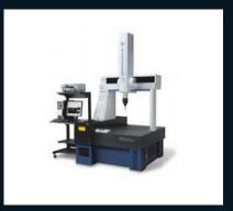
High accuracy CNC coordinate Coordinate Measuring Machine measuring machines capable of 1.7+3L/1000, using MCOSMOS software and TP20 & TP200 touch trigger modules. 2 X S574, size - X: 505mm. Y: 705mm. Z: 405mm
